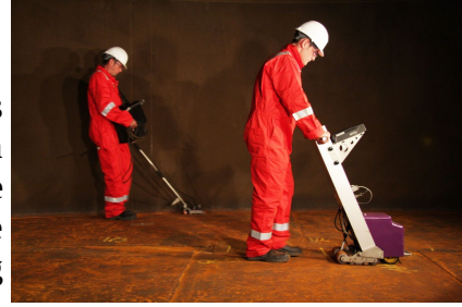
Figure 3: 2 technicians using MFL scanners inside an AST: the smaller handscan (left) and the more advanced FM3D (right)
