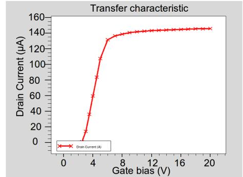
**Fig. 3 Transfer characteristic**
